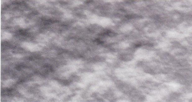
Extrusion haze 10µm
